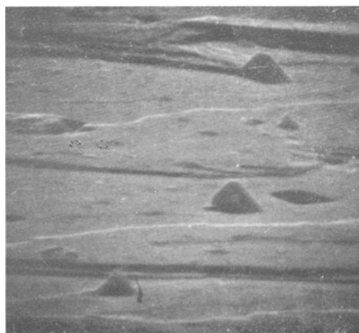
Figure 6 Scanning electron micrograph of the fracture surface of a MgO crystal containing nickel particles, taken at an angle of 10^\circ to the surface.
